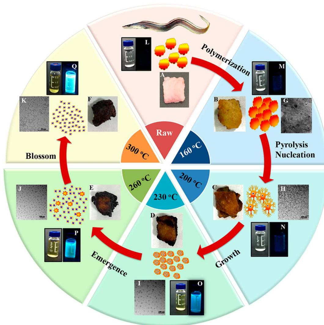
**Fig. 8** A stepwise illustration of the growth and formation mechanism of pike eel-derived N-CDs (red arrow). (A–F) The digital pictures of fish obtained at different roasting temperatures. (G–K) TEM images of corresponding fluorescent materials isolated at various stages. (L–Q) The digital photographs of aqueous soluble CDs under day per UV (365 nm) light. Reprinted (adapted) with permission from ref. 151, Copyright (2018), the American Chemical Society.
