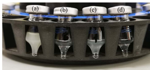
Fig. 6 The physical appearance of the final extractor of nitrofuran metabolites determination, (a) QC (without Hydrophobic CMCs), (b) CMC-C18, (c) CMC-C4, (d) CMC-C1.
