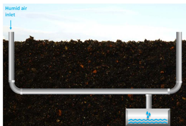
Fig. 13 Schematic of condensation drinking water production method.
