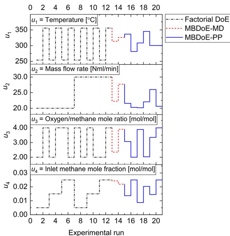
**Fig. 4** Experimental conditions in the factorial, MBDoE-MD and MBDoE-PP campaign of experiments, used by the autonomous platform for identification of an appropriate kinetic model for methane oxidation.
