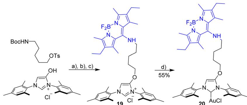
Scheme 6 Synthesis  $[\text{AuCl}(\text{NHC\_blue})]$  **20**. Reagents and conditions: (a)  $\text{K}_2\text{CO}_3$ , KI, acetone, reflux, 12 h; (b) HCl in dioxane,  $\text{CH}_2\text{Cl}_2$ , overnight; (c) meso-Cl-Bodipy,  $\text{Et}_3\text{N}$ ,  $\text{CH}_3\text{CN}/\text{CH}_2\text{Cl}_2$ , 12 h; (d)  $\text{Ag}_2\text{O}$ , DCE,  $T = 60^\circ\text{C}$ , 60 min then  $[\text{AuCl}(\text{SMe}_2)]$ , 12 h.
