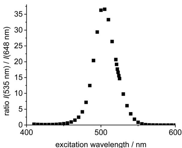
Fig. 2 Plot of excitation wavelength vs. ratio of emission intensities of the individual green Bodipy 11 ( $\lambda_{\text{em,max}} = 535$  nm) and the individual 4 ( $\lambda_{\text{em,max}} = 648$  nm) in DCE ( $c = 5.0 \times 10^{-6}$  mol  $\text{L}^{-1}$ ).
