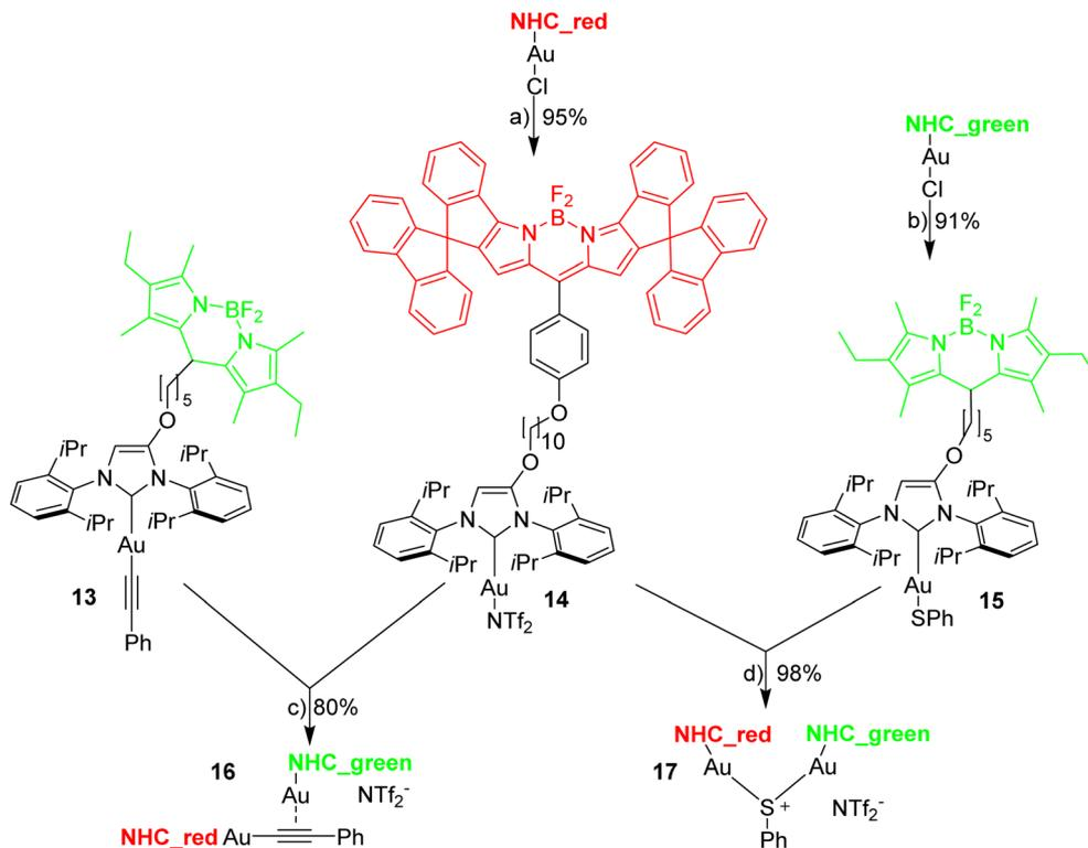
Scheme 4 Synthesis of two red-green dinuclear gold complexes. Reagents and conditions: (a)  $[\text{Au}(\text{NTf}_2)]$ ,  $\text{CH}_2\text{Cl}_2$ , rt, 30 min; (b) 5 equiv. PhSH,  $\text{Et}_3\text{N}$ ,  $\text{EtOH}/\text{CH}_2\text{Cl}_2$ ; (c)  $\text{CH}_2\text{Cl}_2$ , rt, 40 min; (d)  $\text{CH}_2\text{Cl}_2$ , 30 min.
