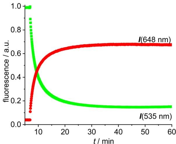
Fig. 3 Time-dependent evolution of the fluorescence (green fluorescence renormalized to 1.0) for the reaction of  $[\text{Au}(\text{CCPh})(\text{NHC\_green})]$  13 with  $[\text{Au}(\text{NTf}_2)(\text{NHC\_red})]$  14 in DCE ( $c = 5.0 \times 10^{-6} \text{ mol L}^{-1}$ ).
