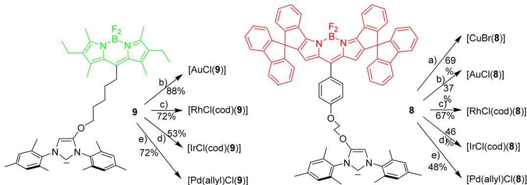
Scheme 2 Synthesis of red and green NHC-metal complexes. Reagents and conditions: (a)–(e) metal source  $[\text{AuCl}(\text{Me}_2\text{S})]$  or  $[\text{RhCl}(\text{cod})]_2$  or  $[\text{IrCl}(\text{cod})]_2$  or  $[\text{Pd}(\text{allyl})\text{Cl}]_2$  or  $[\text{CuBr}(\text{Me}_2\text{S})]$  with  $\text{K}_2\text{CO}_3$ , acetone, reflux, 14 h.
