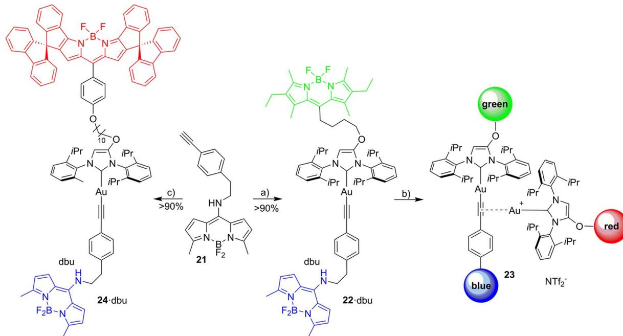
Scheme 8 Synthesis of the blue-green dyad and the blue-green-red triad. Reagents and conditions: (a) [AuCl(NHC\_green)], dbu, CH<sub>2</sub>Cl<sub>2</sub>; (b) + [Au(NTf<sub>2</sub>)(NHC\_red)] **14** in 1,2-dichloroethane; (c) [AuCl(NHC\_red)], dbu, CH<sub>2</sub>Cl<sub>2</sub>.
