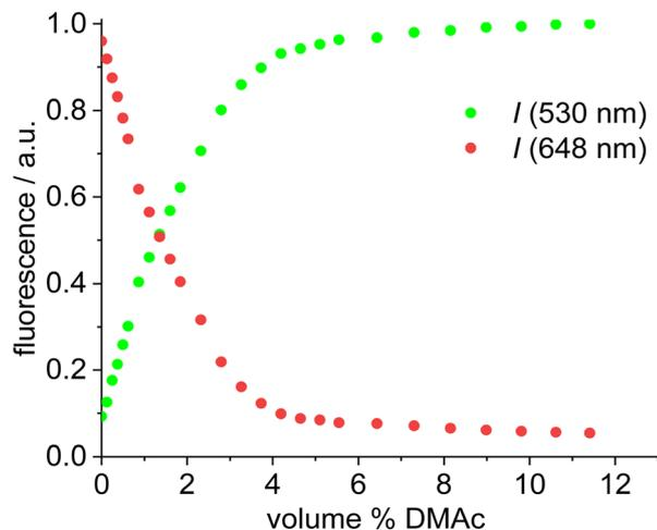
Fig. 6 Plot of the fluorescence of red/green (acceptor/donor) (fluorescence renormalized to 1.0) for complex **19** vs. volume-% of DMAc in toluene solution ( $c = 1.0 \times 10^{-6} \text{ mol L}^{-1}$ ) upon 500 nm excitation.
