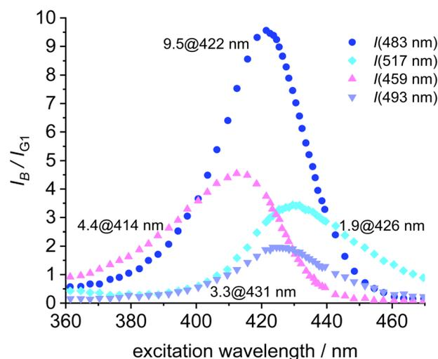
Fig. 8 Plot of the ratio of fluorescence intensities ( $I_B/I_{G1}$ ) vs. the excitation wavelength for **B1**, **B2**, **B3**, **B4** and **G1**. 9.5 @ 422 nm denotes the best ratio  $I(\text{B2})/I(\text{G1})$  at 422 nm excitation for the 483 nm fluorescence ( $c = 2.0 \times 10^{-6} \text{ mol L}^{-1}$ ).
