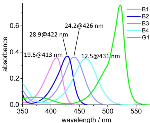
Fig. 7 Absorption spectra of **B1**, **B2**, **B3**, **B4** and the green dye **G1**. The numbers on top of the peaks denote the ratio of the absorption of **B1**, **B2**, **B3** and **B4**, respectively, relative to the absorbance of **G1** at the given wavelengths ( $c = 2.0 \times 10^{-6} \text{ mol L}^{-1}$ ).
