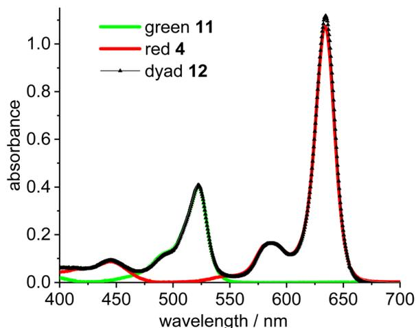
Fig. 1 Absorbance spectra of green Bodipy 11 ( $\lambda_{\text{max}} = 523$  nm) and red Bodipy 4 ( $\lambda_{\text{max}} = 635$  nm) and dyad 12 in  $\text{CH}_2\text{Cl}_2$  ( $c = 5.0 \times 10^{-6}$  mol  $\text{L}^{-1}$ ).
