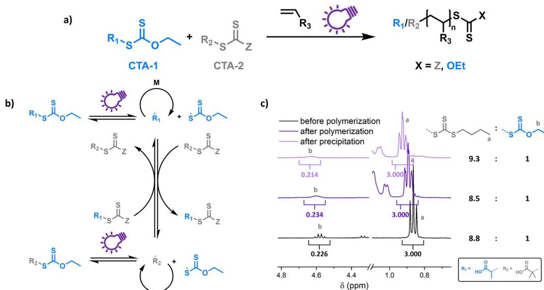
Fig. 1 Schematic representation of XPI-RAFT polymerization (a), and the underlying transfer mechanism from xanthate to CTA-2 (chain transfer between CTAs of equal nature and photo-activation of CTA-2 is not pictured) (b), as well as end group distribution before and after polymerization of a PNAM<sub>10</sub> using a 9 : 1 mixture of CTA-2 (BABTC) and Xan as monitored by <sup>1</sup>H-NMR spectroscopy (c).
