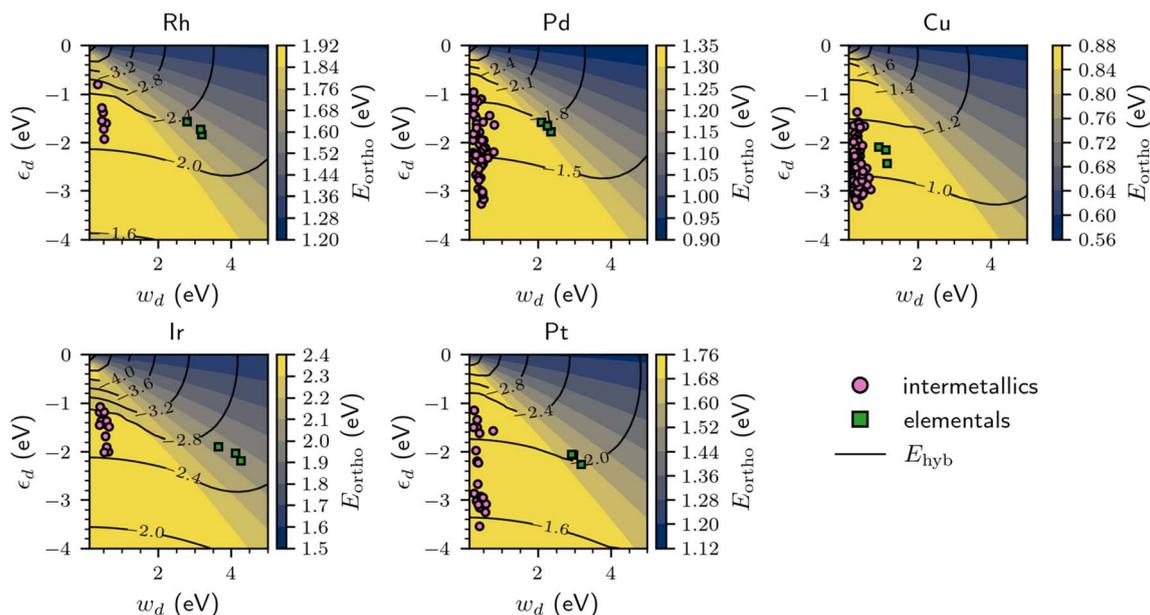
Fig. 5 Orthogonalization energy penalty,  $E_{\text{ortho}}$  (colormap), and hybridization energy,  $E_{\text{hyb}}$  (contour lines), when freely varying the d-band center,  $\epsilon_d$ , and d-band width,  $w_d$ , for different materials considered in this study. The points are from semi-elliptical fits to the d-projected DOS of the metal binding sites on the surface of intermetallics (pink circles) and corresponding transition metals (green squares).
