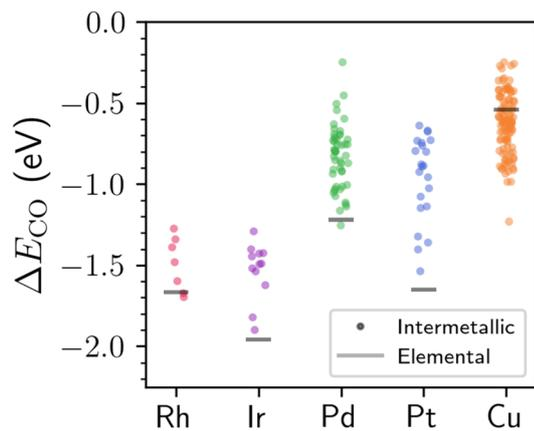
Fig. 4 Adsorption energies,  $\Delta E_{\text{CO}}$ , for CO on the atop site of a given metal with localized d states. Each point represents the CO adsorption process on a material with a different composition and/or surface facet. The points are jittered horizontally for ease of visualization. The horizontal lines represent the average CO adsorption energy at the atop site for the (100), (110), and (111) surfaces of the corresponding ground-state, elemental reference structure.
