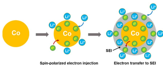
Fig. 4 Schematic illustrations of lithium storage in metallic Co via a spin-polarized electron injection to the 3d orbital of Co and subsequent electron transfer to the surrounding SEI at lower potential.
