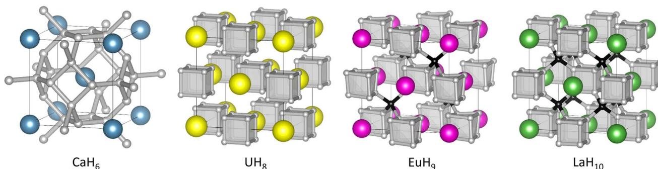
Fig. 1 Structures of high-pressure hydrides  $\text{CaH}_6$ ,  $\text{UH}_8$ ,  $\text{EuH}_9$ , and  $\text{LaH}_{10}$ . In  $\text{EuH}_9$  and  $\text{LaH}_{10}$ , grey and black spheres represent H atoms in cube and tetrahedral sites respectively.
