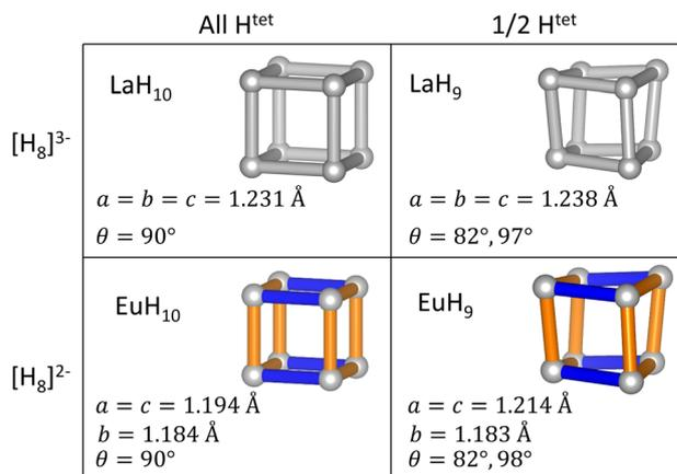
Fig. 5 Geometries of  $H_8$  clusters in  $MH_9$  and  $MH_{10}$  ( $M = La, Eu$ ) arranged by the formal charge on  $H_8$  and the occupancy (full or half) of the  $H^{tet}$  sites. Bond lengths and angles are calculated at 150 GPa. H is shown in grey, La in green, and Eu in pink. Orange and blue bonds denote elongated and compressed H–H bonds respectively.
