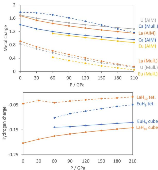
Fig. 2 Upper: computed charges of metal atoms in CaH<sub>6</sub> (blue), LaH<sub>10</sub> (orange), UH<sub>8</sub> (grey) and EuH<sub>9</sub> (yellow) vs. pressure. AIM charges are shown by solid lines, and Mulliken charges by dashed lines. Lower: AIM atomic H charges in EuH<sub>9</sub> (blue) and LaH<sub>10</sub> (orange) resolved into cube (solid line) and tetrahedral (dashed line) atoms.
