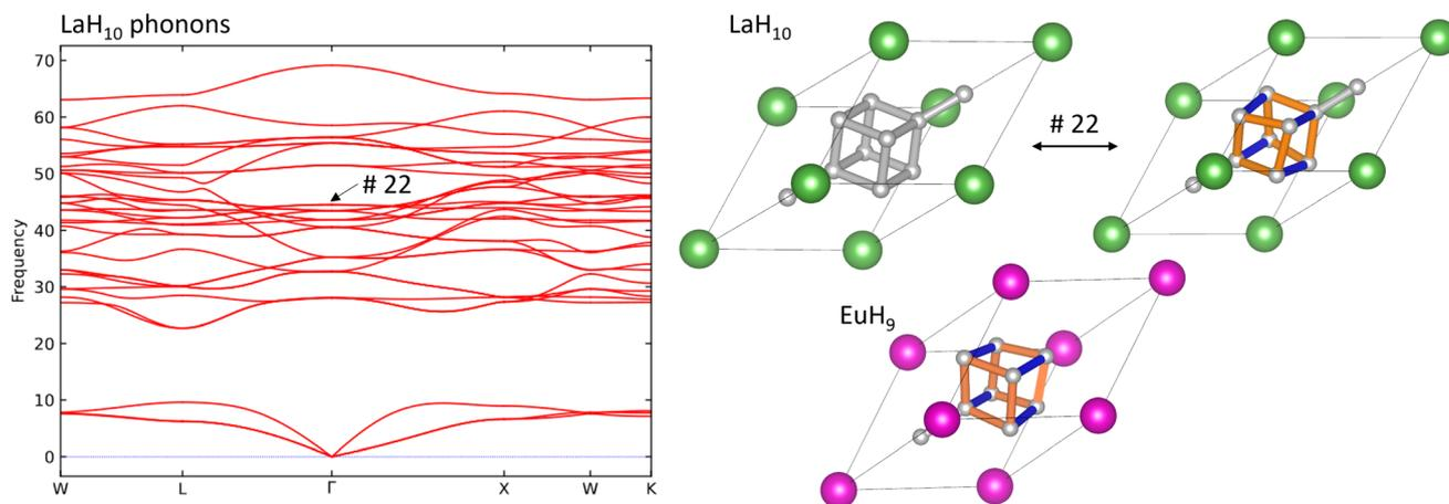
Fig. 6 L: phonon band structure of  $\text{LaH}_{10}$  at 300 GPa. R: undistorted and distorted primitive unit cells of  $\text{LaH}_{10}$ , where the distortion is over mode 22, and the optimized structure of  $\text{EuH}_9$ . La atoms are shown in green, Eu in pink, and H in grey. Orange and blue bonds denote elongated and compressed H–H bonds respectively.
