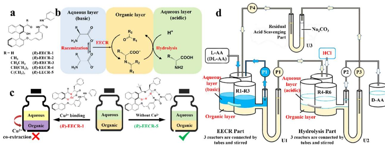
Fig. 3  $\text{Cu}^{2+}$  sequestration and EECR in continuous flow. (a) Carbonyl compounds studied for EECR in this work. (b) Enantioselective extraction coupled with racemization (EECR). (c) Schematic representation of the results using (R)-EECR-1 or (R)-EECR-5 as the extractant. (d) Schematic design of a continuous reaction system that carries out EECR and hydrolysis reactions repeatedly.<sup>53</sup>
