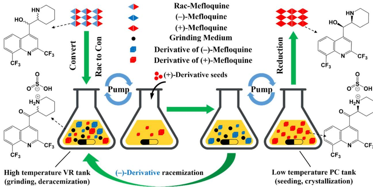
Fig. 17 Experimental chemical derivatization-VR-PC coupled setup used for the deracemization of mefloquine.<sup>262</sup> Blue arrows: crystal-free liquid exchange through tubes.
