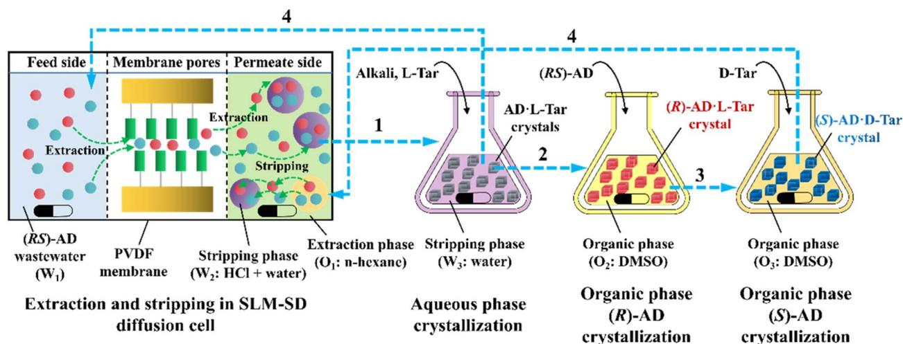
Fig. 32 Schematic diagram of the integrated supported liquid membrane-aqueous/organic phase crystallization separation process (step 1: transfer of  $W_2$  from SLM-SD, step 2: transfer of aqueous phase crystal from  $W_3$ , step 3: transfer of the mother liquor from  $O_2$ , and step 4: mother liquor recycling routes of  $O_3 \rightarrow O_1$  and  $W_3 \rightarrow W_1$ ).<sup>341</sup>
