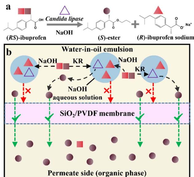
Fig. 31 (a) Coupled strategy of membrane-enhanced enzymatic kinetic resolution by *Candida lipase* and (b) schematic representation of gravity-driven penetration of the reaction mixture through SiO<sub>2</sub>/PVDF membranes.<sup>340</sup>
