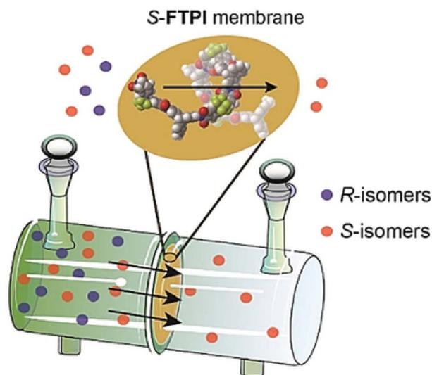
Fig. 27 Schematic representation of triptycene-based chiral porous polyimides for enantioseparation.<sup>326</sup> Reproduced with permission from ref. 326. Copyright 2021, John Wiley and Sons.
