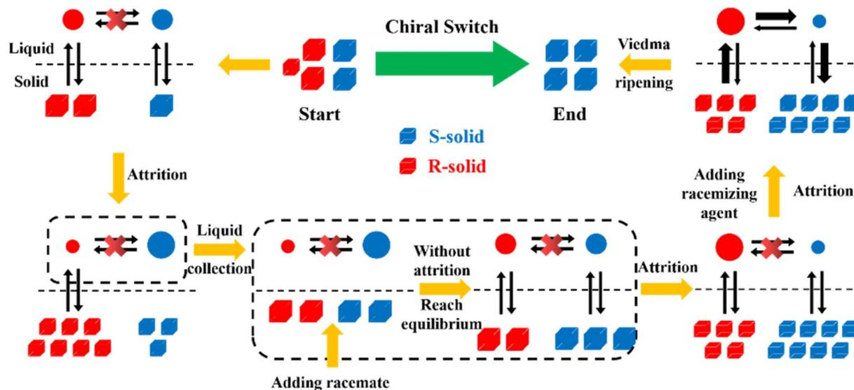
Fig. 16 Stepwise schematic illustration of the "chiral switch" approach.<sup>261</sup>
