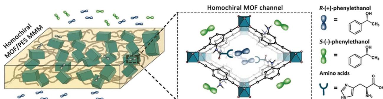
Fig. 26 Schematic illustration of the selective transport of *R*-(+)- and *S*(-)-1-phenylethanol through the MIL-53-NH-*L*-His channel.<sup>325</sup> Reproduced with permission from ref. 325. Copyright 2019, John Wiley and Sons.
