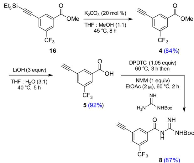
Scheme 2 Sequence used to prepare terminal alkyne 8.
