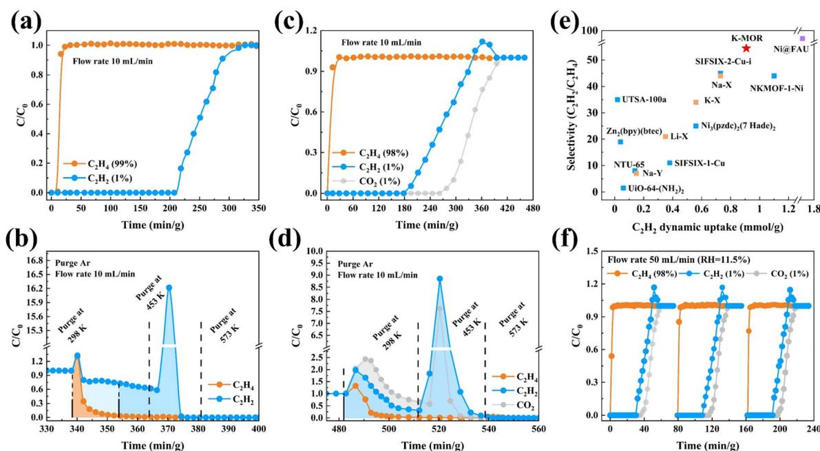
Fig. 4 (a and b)  $\text{C}_2\text{H}_2/\text{C}_2\text{H}_4$  (1/99, v/v) and (c and d)  $\text{CO}_2/\text{C}_2\text{H}_2/\text{C}_2\text{H}_4$  (1/1/98, v/v/v) breakthrough experiments at 298 K. (e) Comparison of  $\text{C}_2\text{H}_2/\text{C}_2\text{H}_4$  dynamic selectivity against  $\text{C}_2\text{H}_2$  dynamic uptake under ambient conditions with a state-of-the-art adsorbent. (f) Cycling breakthrough tests on K-MOR under humid conditions ( $\text{RH} = 11.5\%$ ).
