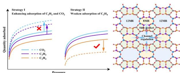
Fig. 1 Diffusion channel regulation strategy for  $CO_2/C_2H_2/C_2H_4$  separation.
