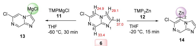
Scheme 4 Thermodynamically driven regioselectivity switch in the metalation of 6-chloroimidazo[1,2-a]pyrazine using either TMPMgCl·LiCl (11) or TMP 2 Zn·2MgCl 2 ·2LiCl (12). Salts are omitted for clarity.
