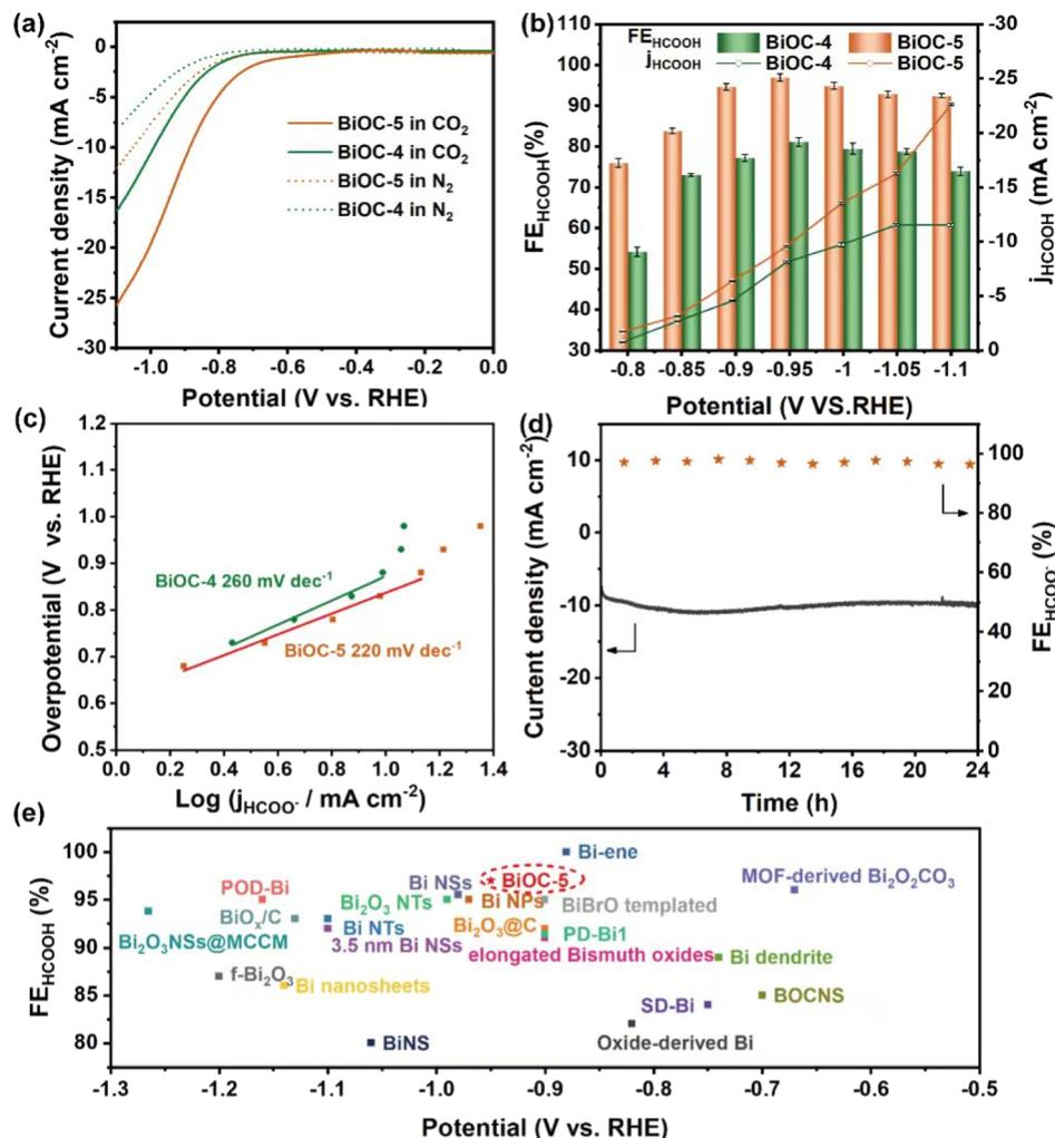
Fig. 2 (a) Polarization curves of BiOC-4 and BiOC-5 in  $N_2$  or  $CO_2$  saturated 0.5 M  $KHCO_3$ . (b) Faradaic efficiencies of production and the current densities of formate at different working potentials in a  $CO_2$ -saturated 0.5 M  $KHCO_3$  electrolyte for BiOC-4 and BiOC-5. (c) Nyquist plots for BiOC-4 and BiOC-5. (d) Stability test of BiOC-5 at  $-0.95$  V vs. RHE for 24 h. (e) Comparison of  $FE_{HCOOH}$  with previously documented reports.
