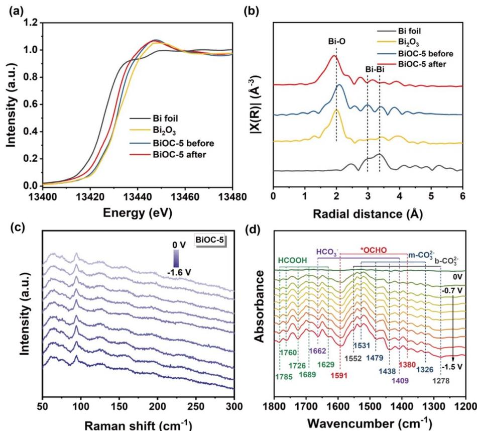
Fig. 3 (a) Bi L3-edge XANES spectra of Bi foil,  $\text{Bi}_2\text{O}_3$ , BiOC-5 before and BiOC-5 after. (b) EXAFS in R-space for Bi foil,  $\text{Bi}_2\text{O}_3$ , BiOC-5 before and BiOC-5 after. (c) *In situ* Raman spectra of  $\text{CO}_2$  reduction on BiOC-5. (d) *In situ* ATR-FTIR spectra of BiOC-5 during the ECR.
