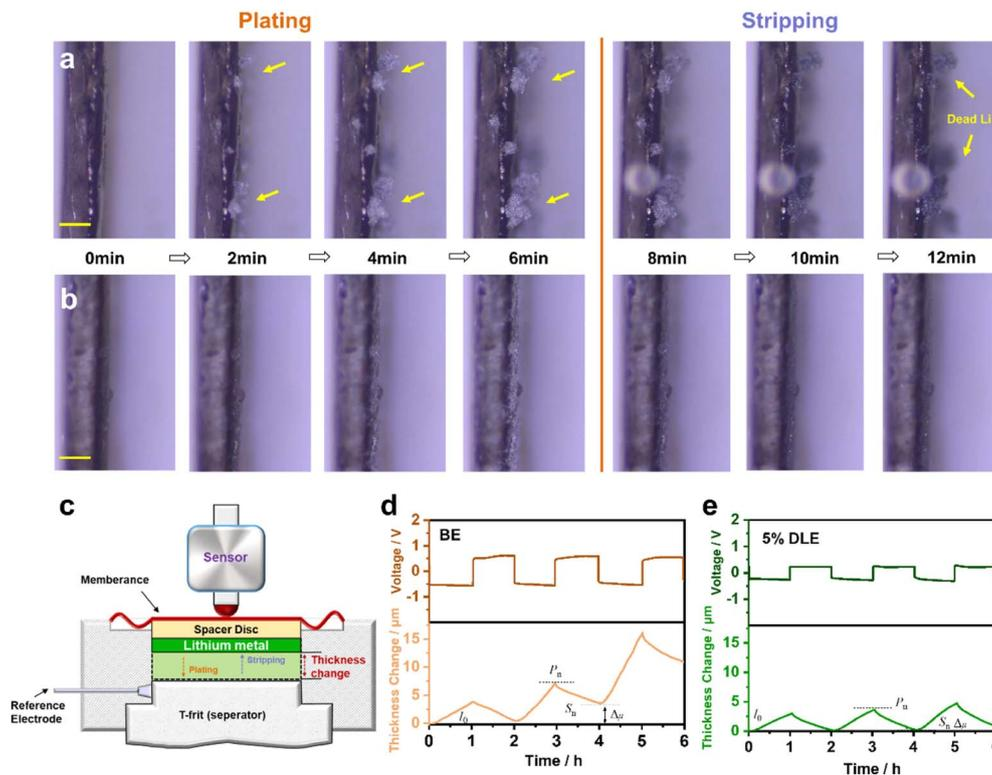
Fig. 2 *In situ* optical microscopy observation of the Li deposition process in (a) the base electrolyte and (b) 5% DLE electrolyte at  $5 \text{ mA cm}^{-2}$  and  $0.5 \text{ mA h cm}^{-2}$ , the ruler is  $200 \mu\text{m}$ . (c) The schematic of the *in situ* electrochemical dilatometry measurement and the thickness change of the lithium anode in (d) the base electrolyte and (e) 5% DLE at the current density of  $1 \text{ mA cm}^{-2}$  for 1 mA h.
