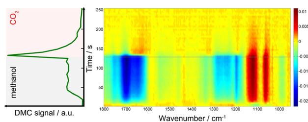
Fig. 1 (left) MS signal of DMC ( $m/z = 59$ ) and (right) time-resolved DRIFT spectra taken during methanol (the first half period) *vs.* CO<sub>2</sub> (the second half period) concentration perturbation experiment performed at 120 °C at 7 ml min<sup>-1</sup>. The time-axes ( $y$ -axis) of both figures are identical. The DRIFT spectra were calculated taking the last spectrum in the CO<sub>2</sub> atmosphere as background.
