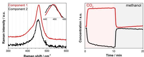
Fig. 3 Multivariate spectral analysis applied for F<sub>2g</sub> band of CeO<sub>2</sub> during DMC synthesis experiment (CO<sub>2</sub> vs. methanol) at 140 °C. The Raman measurement was performed with a 532 nm laser (green). Both spectra (left) and concentration (right) profiles are normalized for clarity.
