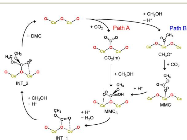
Fig. 4 Reaction mechanism of DMC formation from CO<sub>2</sub> and methanol. Path A starts with an adsorbed CO<sub>2</sub> molecule while Path B starts from the dissociative adsorption of a methanol molecule.
