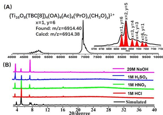
Fig. 4 (A) Positive-mode MALDI-TOF-MS spectrum depicting  $\text{Ti}_{16}\text{L}_{4-1}$  in  $\text{CHCl}_3$  solution; (B) PXRD patterns of  $\text{Ti}_{16}\text{L}_{4-1}$  acquired during acid- and base-stability assessments. Remarkably,  $\text{Ti}_{16}\text{L}_{4-1}$  exhibits robustness even after prolonged exposure to 1 M HCl,  $\text{HNO}_3$ ,  $\text{H}_2\text{SO}_4$ , and 20 M NaOH for 24 hours.
