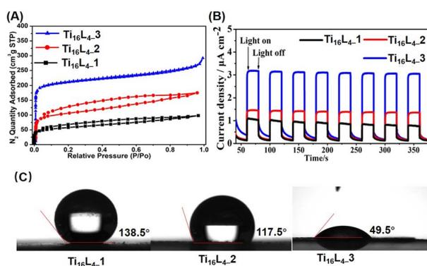
Fig. 3 (A)  $\text{N}_2$  adsorption/desorption isotherm recorded at 77 K; (B) transient photocurrent responses of  $\text{Ti}_{16}\text{L}_4$  captured during Xe lamp irradiation in a 0.2 M  $\text{Na}_2\text{SO}_4$  electrolyte solution; (C) comparative assessment of the wettabilities across  $\text{Ti}_{16}\text{L}_{4-1}$ ,  $\text{Ti}_{16}\text{L}_{4-2}$  and  $\text{Ti}_{16}\text{L}_{4-3}$ .
