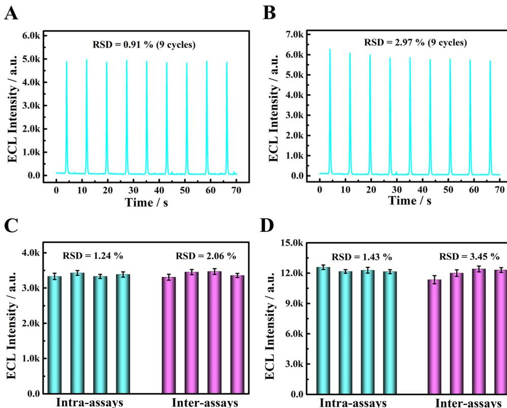
**Fig. 6** Operational stability of the sensor in the case of (A)  $3.0 \times 10^{-5}$  M DA and (B)  $5.0 \times 10^{-5}$  M NE. Reproducibility of the sensor in the case of (C)  $1.0 \times 10^{-4}$  M DA and (D)  $1.0 \times 10^{-8}$  M NE. Detection conditions: potential scanning range of 0–+1.25 V, scan rate of  $0.30 \text{ V s}^{-1}$ , amplifier series of 4 and PMT potential of 700 V.
