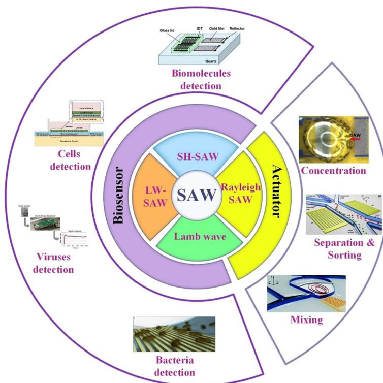
Fig. 1 The SAW devices for biological applications.
