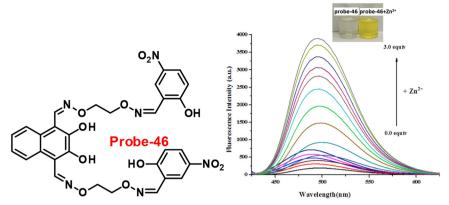
Fig. 62 Chemical structure of probe-46 (left) and changes in the fluorescence spectra of probe-46 upon increasing the Zn(II) ion concentration (right) (reprinted with permission from ref. 106, Copyright 2019 Elsevier).
