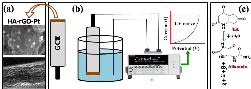
Fig. 9 Schemes of the sensor probe modification and detection of UA via electrochemical investigation. The modification of GCE with HA-rGO-Pt includes layered deposition of the composite, which was confirmed from the SEM image (a); the instrumentation involves the assembly of a two-electrode system for *I-V* analysis (b); the detection of UA involves signal generation due to its electron transfer reaction to produce allantoin (c).
