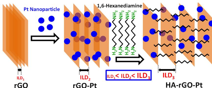
**Fig. 1** Scheme of the synthesis of the HA-rGO-Pt composite. Two principal steps were followed to synthesize the material. In the first step, GO was mixed with HPtCl<sub>4</sub> in an aqueous system. In the second step, the GO-Pt was mixed with HA and subsequently reduced using hydrazine solution. The ILD gradually increases from rGO to rGO-Pt to HA-rGO-Pt.
