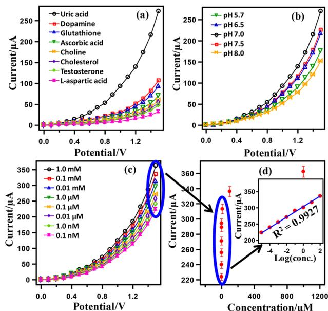
Fig. 4 The electrochemical detection of UA using the HA-rGO-Pt-GCE sensor probe. Analysis of a series of biomolecules to identify selectivity (a); detection of 0.1  $\mu$ M UA at various pH values (b); *I*-*V* responses for various concentrations of UA at pH 7 (c); current vs. concentration of UA at a fixed potential of 1.5 V (d); respective current vs. log (conc.) profile (inset of (d)).
