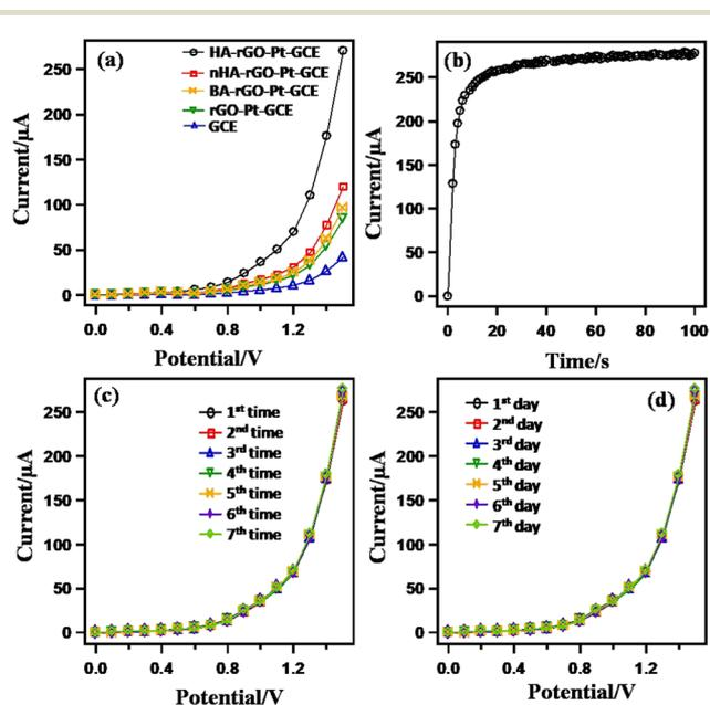
Fig. 5 Control experiments for the UA sensor through monitoring the  $I$ - $V$  response in  $0.1 \mu\text{M}$  UA (7.0 pH buffer). Bare and modified GCE (a); varied response time (b); reusability (c); and (d) stability.
