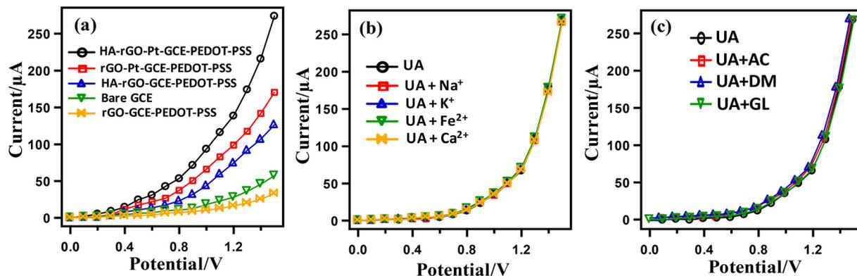
Fig. 6 Effect of the substrate and interfering species. Current response of HA-rGO-Pt-GCE and other substrates in 0.1  $\mu\text{M}$  UA solution (a); interference of common electrolytes (b); and interference of organic species including glucose (GL), ascorbic acid (AC) and dopamine (DM) (c).
