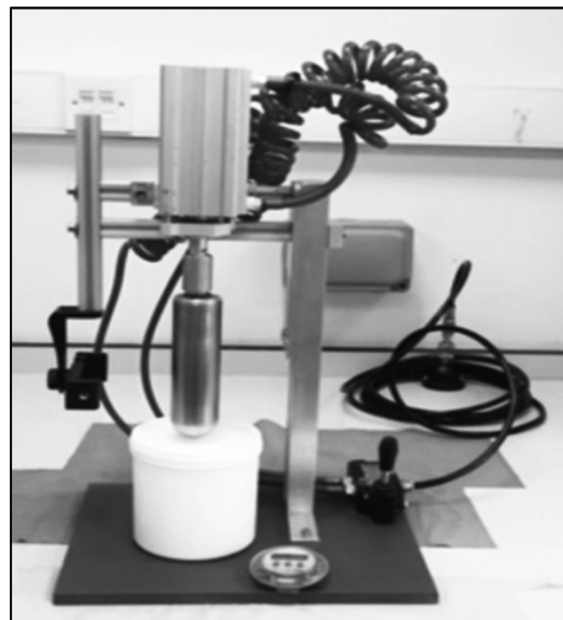
Fig. 3 Apparatus for static dipping used for coagulant leakage experiments. The cylindrical former with hemispherical end is made of stainless steel and it is lowered into the latex vessel pneumatically and then, after a set dwell time, withdrawn with a velocity of 0.076 m s -1 .
