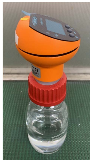
Fig. 3 Commercial biodegradability measuring machine.
