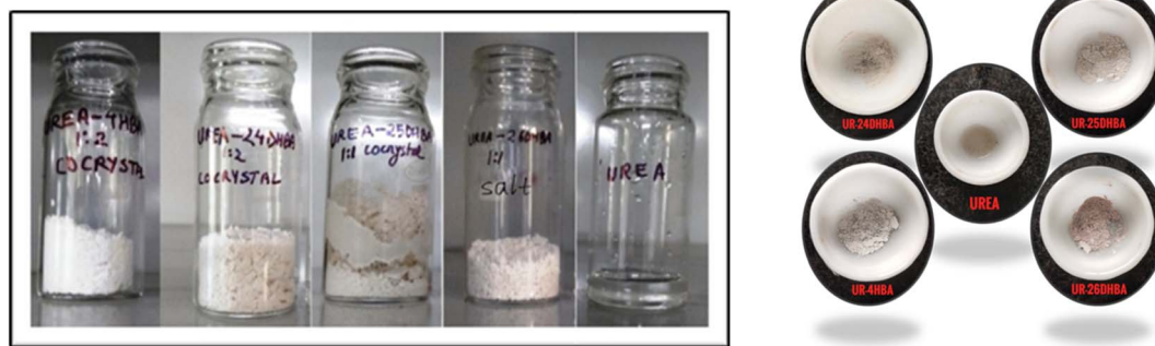
Fig. 3 (Left) Comparison of solubilities for urea·4HBA, urea·24DHBA, urea·25DHBA, urea·26DHBA with pure urea under controlled experiments; (Right) powder samples of urea and respective hydroxybenzoic acid cocrystals/salt stored under 75% RH and ambient temperature. All the multicomponent solids remain as powders without showing deliquescence behaviour even after a period of 2 months, whereas urea deliquesces after a period of ~1.5 months.
