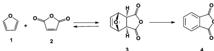
Fig. 21 Reaction path to produce biobased phthalic anhydride as elaborated by Mahmoud and co-workers.<sup>633</sup>
