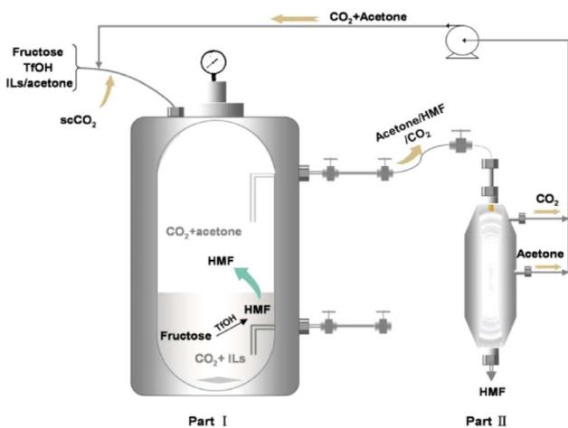
Fig. 12 System of Shi and co-workers for the extraction of HMF from ionic liquids with a mixture of acetone and CO<sub>2</sub> with continuous concentration.<sup>303</sup>
