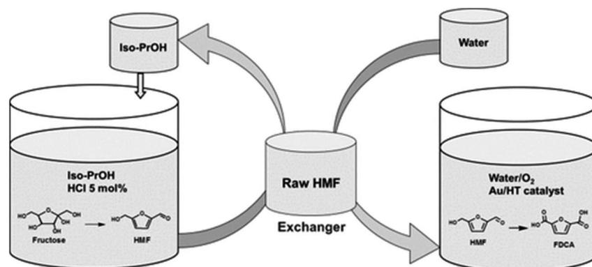
Fig. 17 Two-step process reported by Yi and co-workers for the synthesis of FDCA from fructose.<sup>524</sup>
