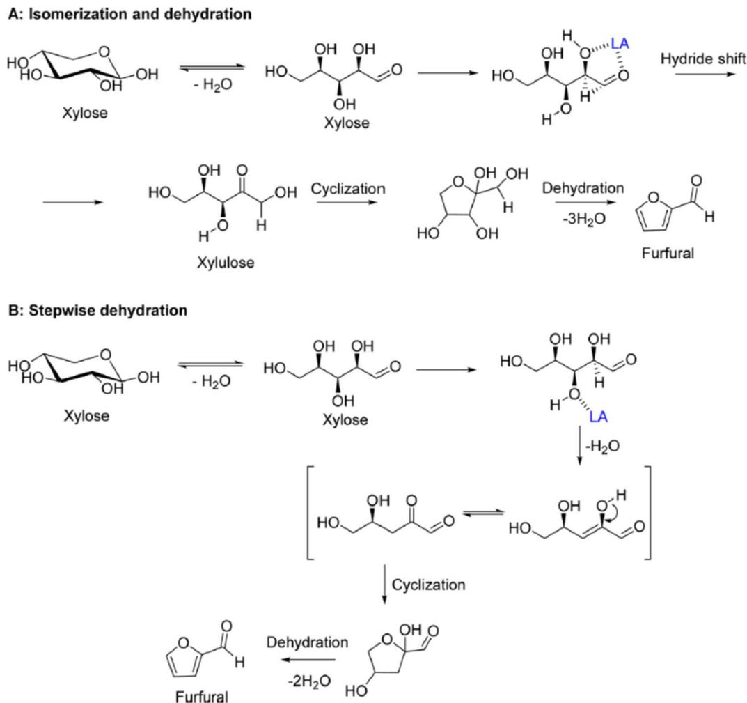
Fig. 13 Reaction mechanisms proposed by Gupta and co-workers<sup>396</sup> for the synthesis of furfural using homogeneous (A) and heterogeneous Lewis acids (B).
