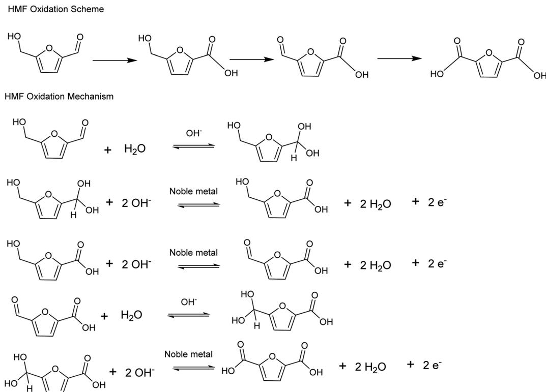
Fig. 14 Reaction scheme proposed by Davis and co-workers for the oxidation of HMF into FDCA passing through geminal diols.<sup>435</sup>
