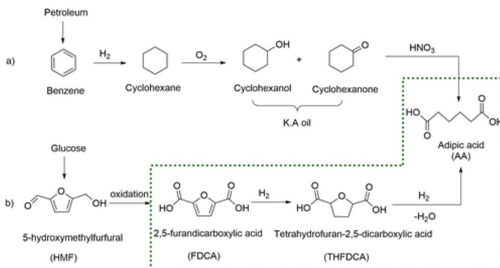
Fig. 18 Catalytic path to produce adipic acid using FDCA as substrate. Reported by Baek and co-workers.<sup>576</sup>
