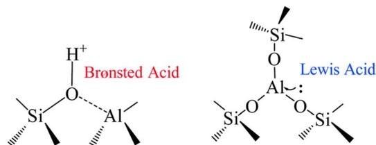
Fig. 10 Brønsted and Lewis acid sites in silicoaluminate catalysts.<sup>250</sup>
