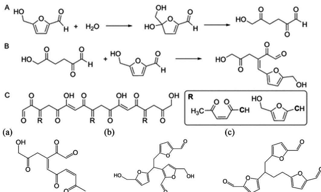
Fig. 6 Proposed scheme and by-products of HMF degradation in water.<sup>78,105</sup>
