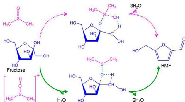
Fig. 8 Mechanism of fructose dehydration into HMF in DMSO.<sup>119</sup>
