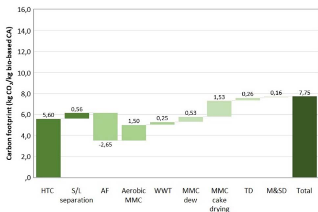
Fig. 5 Carbon footprint estimate for 1 kg of bio-based CA, absolute value and breakdown by main life cycle stage. Own calculation based on chemical plant modelling at the semi-pilot scale. 31 HTC – hydrothermal carbonization; S/L – solid/liquid separation; AF – anaerobic fermentation; MMC – mixed microbial cultures; WWT – wastewater treatment; TD – thermolytic distillation; M & SD – monitoring and safety design.
