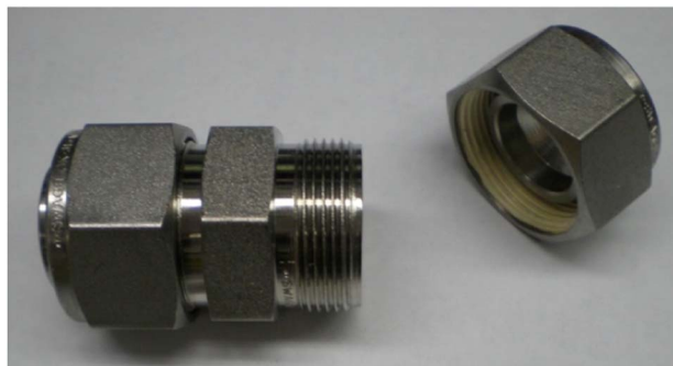
Fig. 5 Photograph of 10 mL mini-reactors built from Swagelok junctions. (Figure from ref. 27, Copyright 2015 American Chemical Society).
