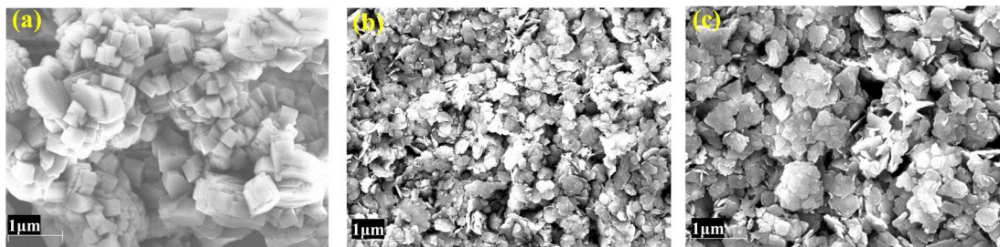
Fig. 2 FE-SEM results of (a) MWW-zeolite (b) Zn(II)-exchanged MWW-zeolite, (c) chiral Zn-salen@MWW.
