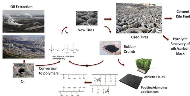
Fig. 1 The automotive rubber tire life cycle.
