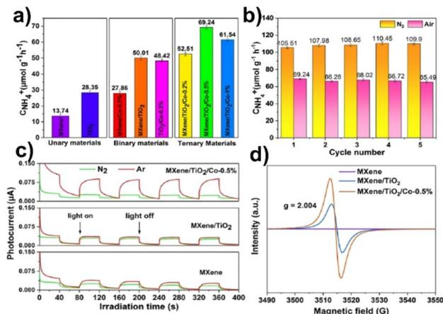
Fig. 12 (a) NH<sub>4</sub><sup>+</sup> production rate in ambient air; (b) the stability of N<sub>2</sub> photofixation activity of MXene/TiO<sub>2</sub>/Co-0.5% under N<sub>2</sub> and an air atmosphere; (c) photocurrent spectra of MXene, MXene/TiO<sub>2</sub> and MXene/TiO<sub>2</sub>/Co-0.5%; (d) EPR spectra. Reproduced with permission from ref. 163, Copyright 2015 American Chemical Society.
