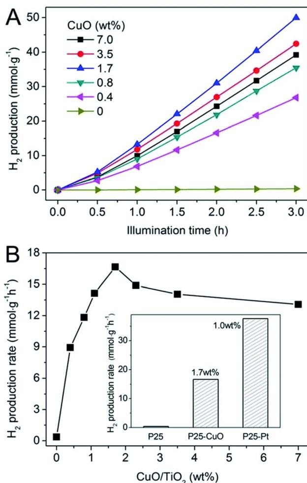
Fig. 16 (A) Hydrogen production vs. illumination time in the presence of CuO-decorated  $\text{TiO}_2$  catalysts. (B)  $\text{H}_2$  production rate vs. loading amount of CuO. The inset of (B) is a bar graph showing the activity of CuO-decorated  $\text{TiO}_2$  in comparison to that of a Pt-decorated system. Reproduced with permission from ref. 191, Copyright 2014 The Royal Society of Chemistry.
