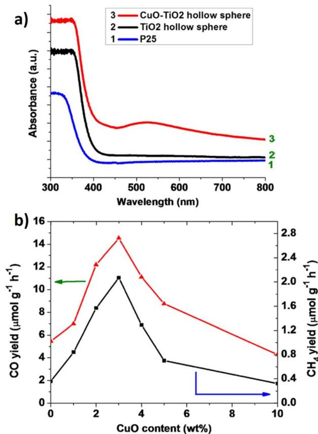
Fig. 17 (a) UV-vis DRS for various TiO<sub>2</sub> based nano-materials. The CuO content in the CuO–TiO<sub>2</sub> catalyst is 3 wt%. (b) Yields of the gas products (CO and CH<sub>4</sub>) produced during 24 h of photo-driven CO<sub>2</sub> reduction on the TiO<sub>2</sub> hollow microsphere catalysts with various Cu contents. Reproduced with permission from ref. 194, Copyright 2015 American Chemical Society.
