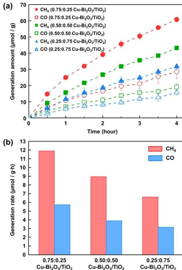
Fig. 18 (a) Amount of CH<sub>4</sub> and CO generated upon using 0.75 : 0.25, 0.50 : 0.50, and 0.25 : 0.75 Cu–Bi<sub>2</sub>O<sub>3</sub>/TiO<sub>2</sub> photocatalysts. (b) Rates of CH<sub>4</sub> and CO generation in the first 4 h of irradiation. Reproduced with permission from ref. 217, Copyright 2016 European Chemical Societies Publishing.
