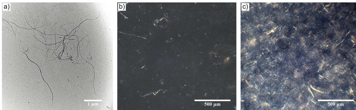
Fig. 1 (a) Transmission electron micrograph (TEM) of CNFs. Cross-polarised optical micrographs of (b) a LiTFSI salt-doped (salt concentration  $r = 0.04$ ) EO-co-EPI electrolyte film without CNFs and (c) the corresponding composite electrolyte film containing 10% w/w CNFs.
