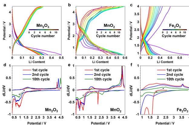
Fig. 6 The first 11 “insertion” cycles of (a)  $\alpha$ - $\text{Mn}_2\text{O}_3$ , (b)  $\beta$ - $\text{MnO}_2$ , and (c)  $\alpha$ - $\text{Fe}_2\text{O}_3$ . The selected derivatives of the 1st (red), 2nd (blue) and 10th (green) cycles are shown below for (d)  $\alpha$ - $\text{Mn}_2\text{O}_3$ , (e)  $\beta$ - $\text{MnO}_2$ , and (f)  $\alpha$ - $\text{Fe}_2\text{O}_3$ . Black arrows indicate the reversible redox pairs.
