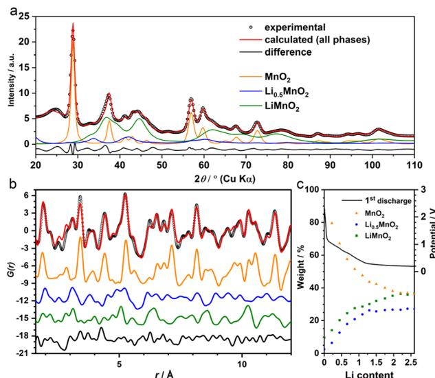
Fig. 3 (a) XRD ( $R_w = 4.5\%$ ) and (b) PDF ( $R_w = 39\%$ ) refinements of the *operando* data at Li 2.0. Calculated patterns from MnO<sub>2</sub> ( $P4_2/mnm$ , orange), Li<sub>0.5</sub>MnO<sub>2</sub> ( $Cmmm$ , blue) and DRX-LiMnO<sub>2</sub> ( $C2/m$ , green) are shown for comparison. (c) The change of their phase ratios during the “insertion” step derived from the PDF refinement.
