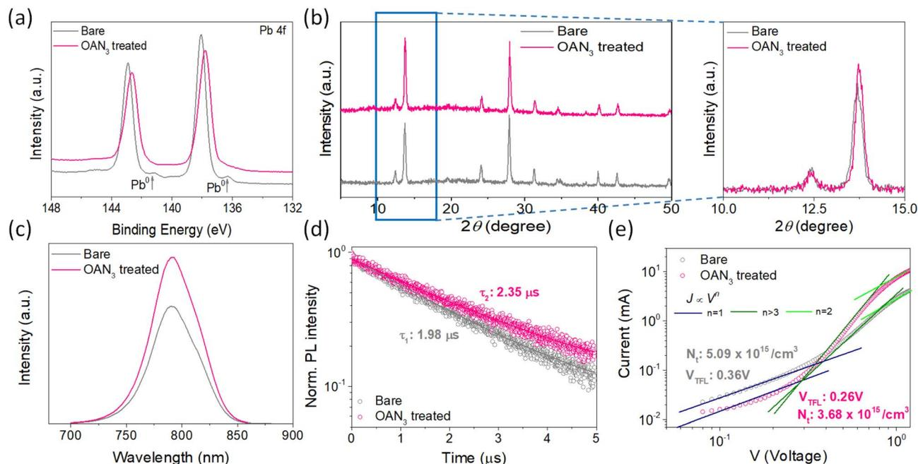
Fig. 3 (a) XPS spectrum of Pb 4f before and after OAN<sub>3</sub> introduction. (b) XRD spectrum of perovskite film under various conditions. (c) Steady-state and (d) time-resolved photoluminescence schematic illustration of perovskite solar cells with and without OAN<sub>3</sub>. (e) Space charge limited current measurement for hole-only devices with and without OAN<sub>3</sub>.
