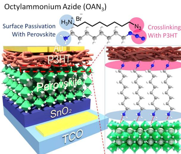
Fig. 1 Schematic illustration of perovskite solar cells with cross-linkable molecule, octylammonium azide (OAN<sub>3</sub>).
