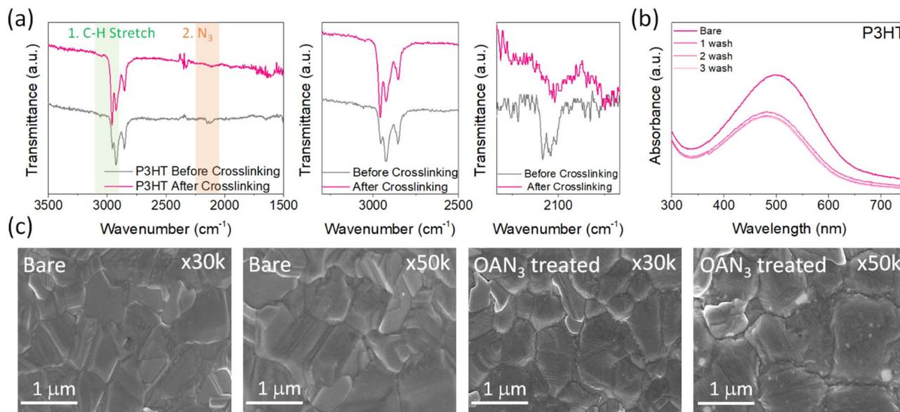
Fig. 2 (a) The FT-IR spectra before and after crosslinking. (b) UV-Vis spectra of P3HT after crosslinking and washing with chlorobenzene. (c) SEM images of perovskite film with different concentrations of OAN<sub>3</sub>.
