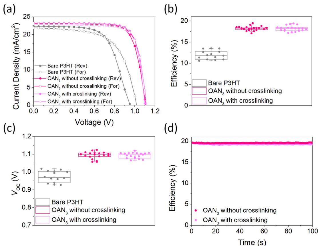
Fig. 4 (a)  $J$ - $V$  curve of champion PSCs before and after OAN<sub>3</sub> introduction. Histogram of (b) power conversion efficiency and (c)  $V_{oc}$  before and after OAN<sub>3</sub> introduction. (d) Stabilized power output before and after OAN<sub>3</sub> introduction.
