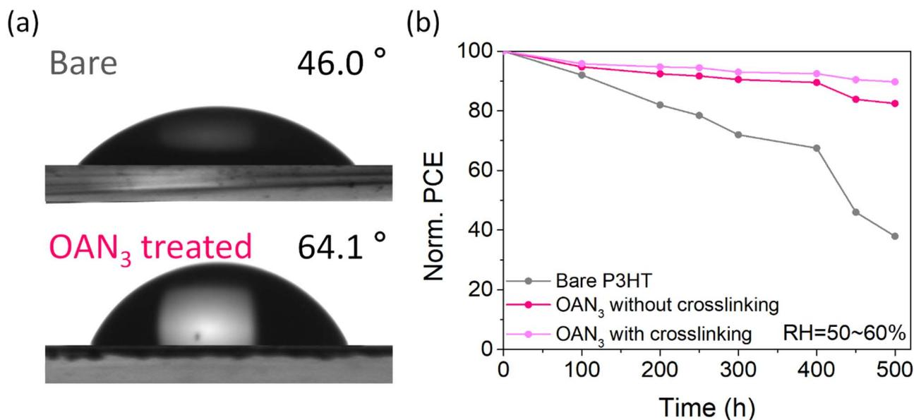
Fig. 5 (a) Contact angles of perovskite film before and after OAN<sub>3</sub> treatment. (b) Moisture-stability under RH: 50–60% storage for PSCs with bare, OAN<sub>3</sub> treated non-crosslinking, and after crosslinking.
