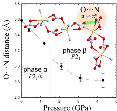
Fig. 7 Distance O...N between adjacent bidentate NO<sub>3</sub>-ligands interacting by a  $\pi^* \leftarrow n$  O...N interaction aggregating adjacent binuclear centers (cf. Fig. S11, ESI†).
