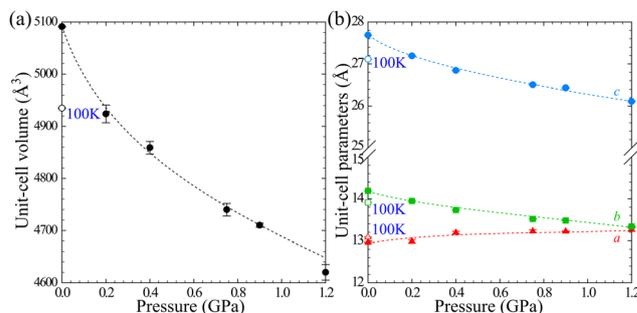
Fig. 9 Compression of Cu(HDA)<sub>2</sub>(MeCN)<sub>2</sub>·2BF<sub>4</sub>: (a) the unit-cell volume; and (b) unit-cell parameters *a*, *b*, and *c*. The open symbols mark the dimensions at 100 K/0.1 MPa. The measurement at 1.2 GPa, due to the reduced reflections intensities caused by the partial amorphization of the sample, provides the unit-cell parameters only.
