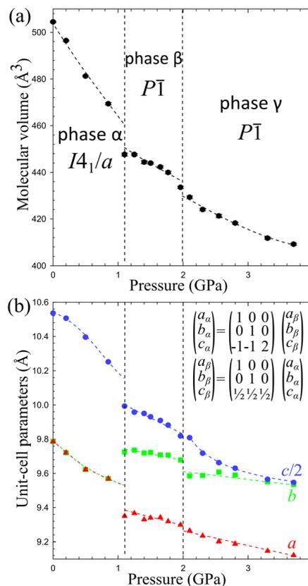
Fig. 2 The unit-cell parameters of crystal  $\text{Cd}(\text{HDA})_2(\text{NO}_3)_2$ , all calculated for the tetragonal setting of phase  $\alpha$  (*cf.* the matrices in Fig. 2(b)) as a function of pressure. The ESD's are smaller than the plotted symbols. The vertical dashed lines mark the critical pressures between the phases. The lines joining the points are for guiding the eye only.
