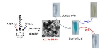
Peroxidase-like Cu-Fe bimetal oxide mesoporous nanospheres identified for the efficient recognition of toxic o-aminophenol and bioactive glutathione
