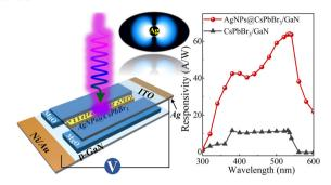
Plasmon-enhanced photoresponse and stability of a CsPbBr<sub>3</sub> microwire/GaN heterojunction photodetector with surface-modified Ag nanoparticles
