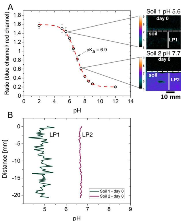
Fig. 4 (A) pH calibration curve showing the  $pK_a$  of the respective pH optode and the dynamic range. Error bars depict the minima and maxima of the chosen regions of interest for each calibration step. (B) Line profiles resulting from Study 1 using Soil 1 ( $pH_{\text{Electrode}}$  5.6), LP1, and Study 2 using Soil 2 ( $pH_{\text{Electrode}}$  7.7), LP2, where no sludge was added in either of the shown images.
