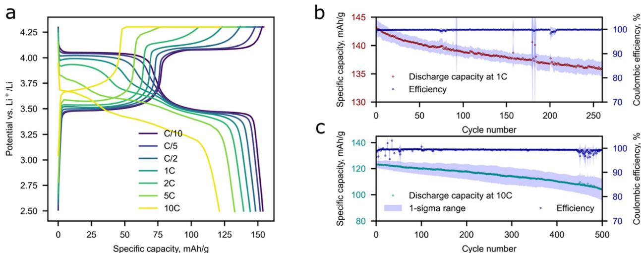
Fig. 5 The electrochemical performance of Li-rich LFMP in Li half-cells. (a) Charge–discharge profiles of Li-rich LFMP at different C-rates, cycling stability of Li-rich LFMP at 1C (b) and 10C (c). The standard deviations (1-Sigma range) and mean values of discharge specific capacity and coulombic efficiency are calculated from five experiments (b and c).
