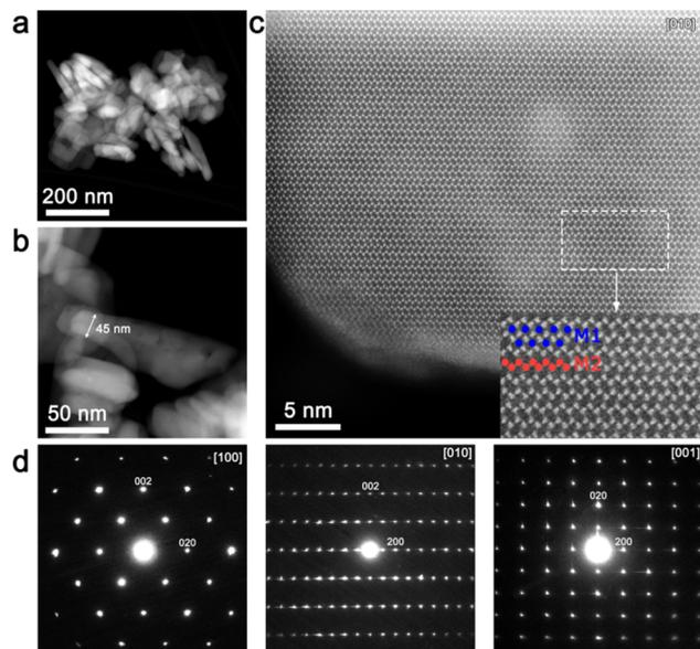
**Fig. 3** (a) An overview and (b) the [100] HAADF-STEM image of Li-rich LFMP particles. The minimal thickness along the *b*-axis (denoted with a double sided arrow) is  $\sim 45$  nm. (c) The low-pass filtered [010] HAADF-STEM image of a Li-rich LFMP crystal; in the magnified area, Fe/Mn atomic columns and Li positions are represented as red and blue circles respectively. (d) The [100], [010] and [001] SAED patterns for Li-rich LFMP.
