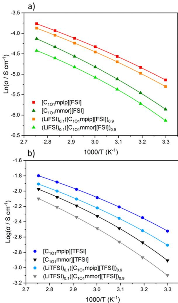
**Fig. 5** Temperature dependent ionic conductivity plots of (a) FSI-based ionic liquids and their 10 mol% LiFSI electrolyte solutions and (b) TFSI-based ionic liquids and their 10 mol% LiTFSI electrolyte solutions.
