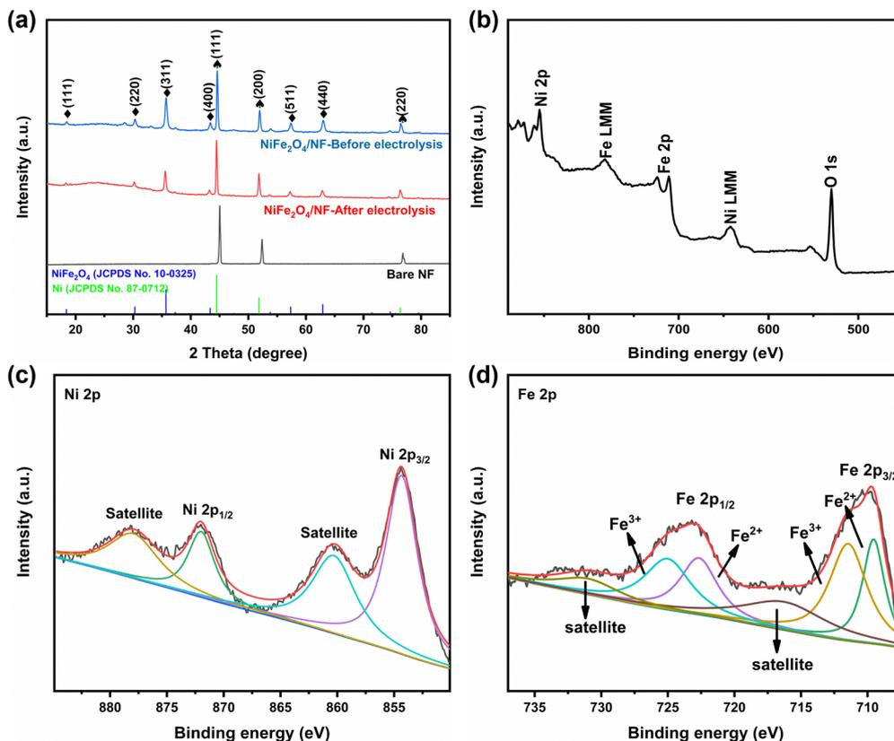
Fig. 3 (a) XRD patterns of NiFe<sub>2</sub>O<sub>4</sub>/NF, (b) XPS survey of NiFe<sub>2</sub>O<sub>4</sub>/NF, and high-resolution XPS of (c) Ni 2p and (d) Fe 2p.
