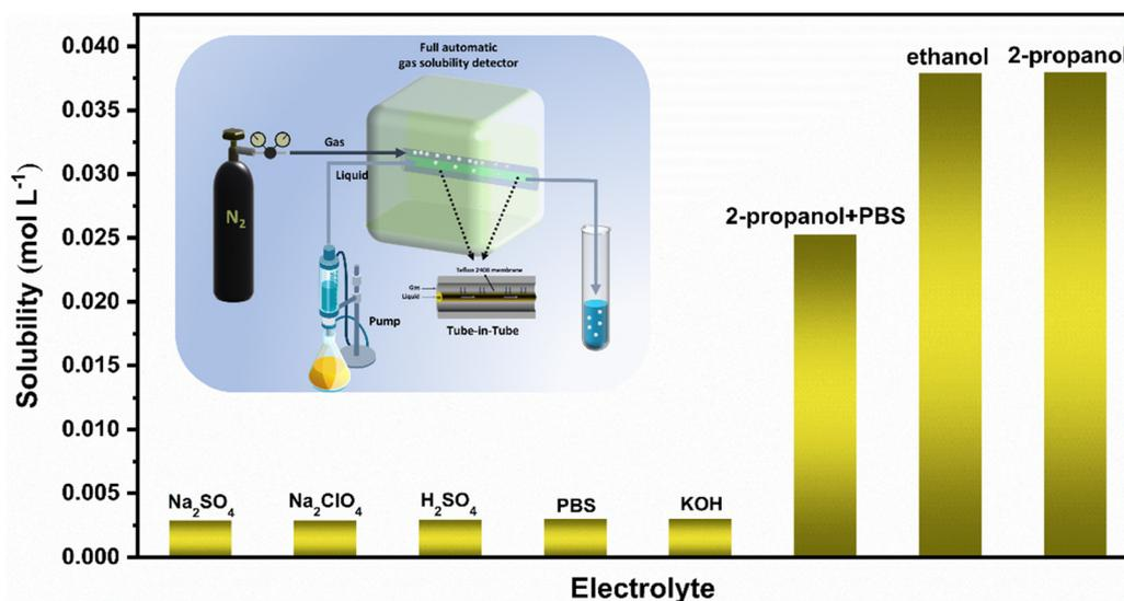
Fig. 1 Solubility of N<sub>2</sub> in different solutions (the illustration shows a schematic diagram of the automatic gas solubility detector).
