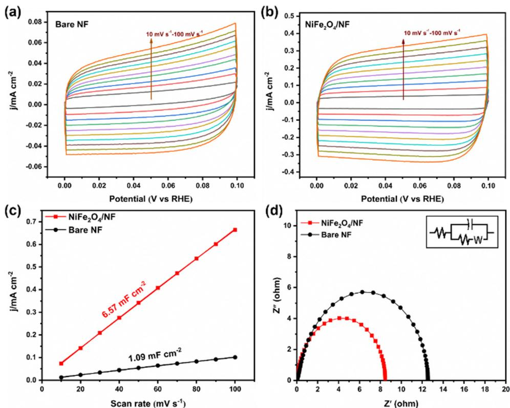
Fig. 5 CV curves of (a) bare NF and (b) NiFe<sub>2</sub>O<sub>4</sub>/NF measured at different scan rates of 10–100 mV s<sup>-1</sup>. (c) The dependence of current density on the potential scan rate for bare NF and NiFe<sub>2</sub>O<sub>4</sub>/NF. (d) EIS plots of bare NF and NiFe<sub>2</sub>O<sub>4</sub>/NF.
