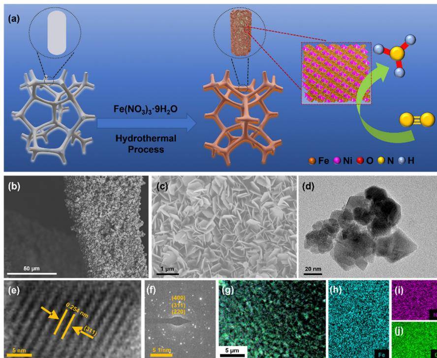
Fig. 2 (a) Scheme of *in situ* growth of  $\text{NiFe}_2\text{O}_4$  nanoarrays on the nickel foam substrate using a hydrothermal method. (b and c) SEM images of  $\text{NiFe}_2\text{O}_4/\text{NF}$ . (d) TEM images of  $\text{NiFe}_2\text{O}_4$  scraped from NF. (e) HRTEM image. (f) The SAED pattern of  $\text{NiFe}_2\text{O}_4$ . (g–j) EDX elemental mapping images of  $\text{NiFe}_2\text{O}_4/\text{NF}$ .
