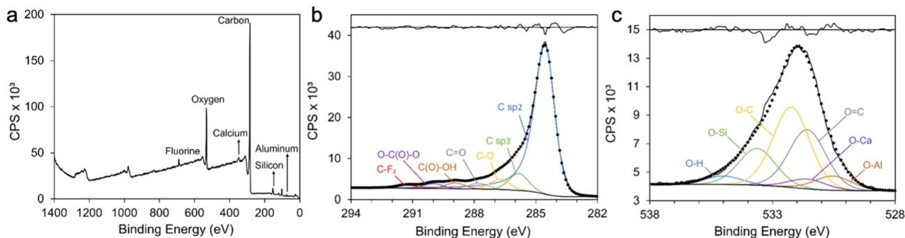
Fig. 3 XPS spectra of coal char including: (a) survey spectra; (b) C1s and (c) O1s narrow scans. Residual standard deviations of peak fittings are provided in (b) and (c) (upper black lines).
