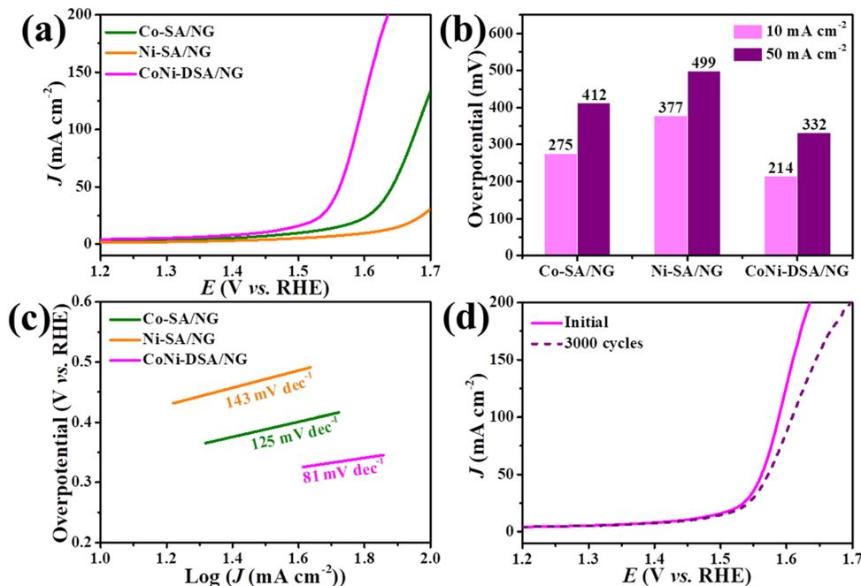
Fig. 5 (a) OER polarization curves, (b) overpotential contrast at the current density of 10 and 50 mA cm<sup>-2</sup>, and (c) Tafel slopes of Co-SA/NG, Ni-SA/NG and CoNi-DSA/NG. (d) The polarization curves before and after 3000 CV of CoNi-DSA/NG (all tested in 1.0 M KOH solution).
