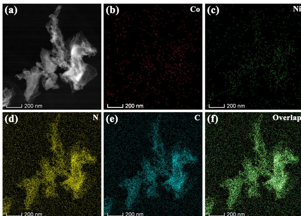
Fig. 2 (a) HAADF-STEM image, EDX elemental mapping of (b) Co, (c) Ni, (d) N and (e) C, and (f) overlap of CoNi-DSA/NG.
