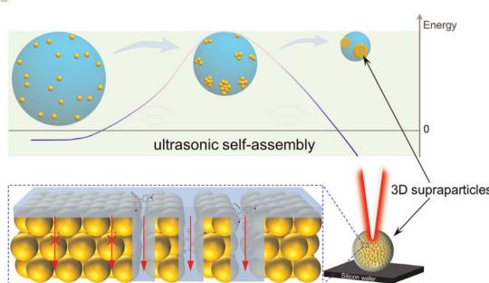
**Ag supraparticles with 3D hot spots to actively capture molecules for sensitive detection by surface enhanced Raman spectroscopy**
