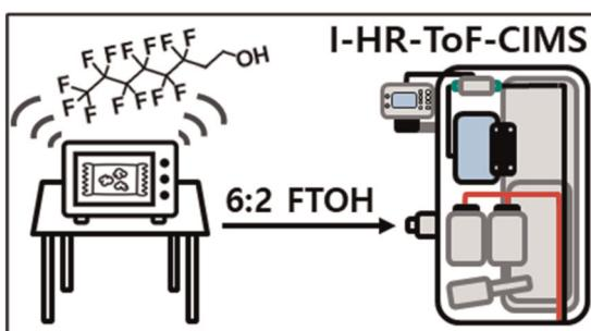
**External liquid calibration method for iodide chemical ionization mass spectrometry enables quantification of gas-phase per- and polyfluoroalkyl substances (PFAS) dynamics in indoor air**
