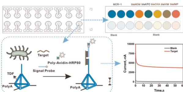
**A multi-channel electrochemical biosensor based on polyadenine tetrahedra for the detection of multiple drug resistance genes**
