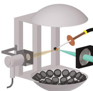
**Elemental analysis of levitated solid samples by microwave-assisted laser induced breakdown spectroscopy**
