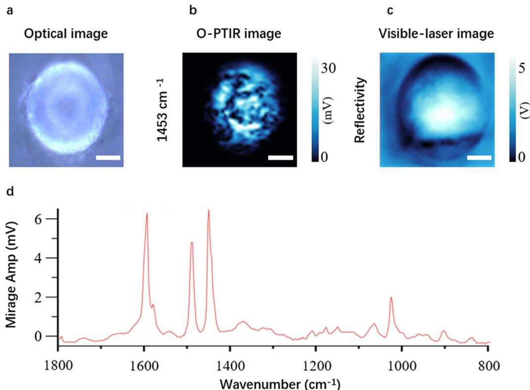
Fig. 2 An optical image (a), a single frequency image at 1453 cm<sup>-1</sup> (b), a visible-laser image (c), and a spectrum of a polystyrene (PS) microbead (d) placed on a glass slide acquired using our in-house mIRage O-PTIR microscope. A single frequency image obtained with the O-PTIR technique is often referred to as an O-PTIR image. 1453 cm<sup>-1</sup> is the band where PS shows one of its characteristic peaks. The white scale bar is 20 μm. The colour scales show the signal intensity.
