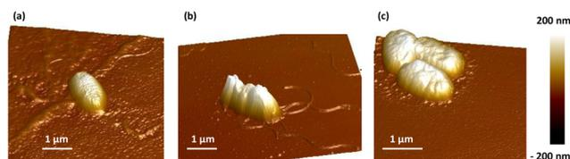
**Fig. 7** PF-QNM surface topography images of *P. aeruginosa* PAO1-Tn7-*gfp* adhering on Fn (1.0 μM) (a), BSA (0.75 μM) (b), and BSA (10.0 μM) (c) dehydrated protein conditioning layers adsorbed on SiO<sub>2</sub> surfaces.
