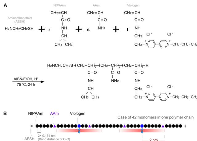
**Fig. 2** Precise design of the ternary copolymer. (A) Preparation of poly(NIPAAm-co-AAm-co-viologen) by telomerization. (B) Schematic of PNAV as a linear chain, calculated with the values in polymer properties.
