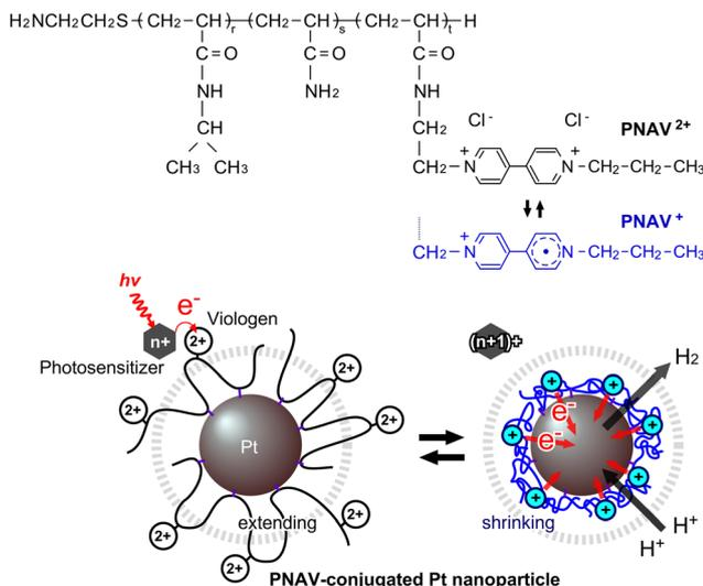
**Fig. 1** Photoinduced H<sub>2</sub> generation system using poly(NIPAAm-co-AAm-co-viologen) (PNAV). Chemical structure and redox states of PNAV and electron transfer driven by coil-globule transitions of PNAV conjugated on Pt nanoparticles (NPs). The dot circle means the effective distance from the Pt NP surface.
