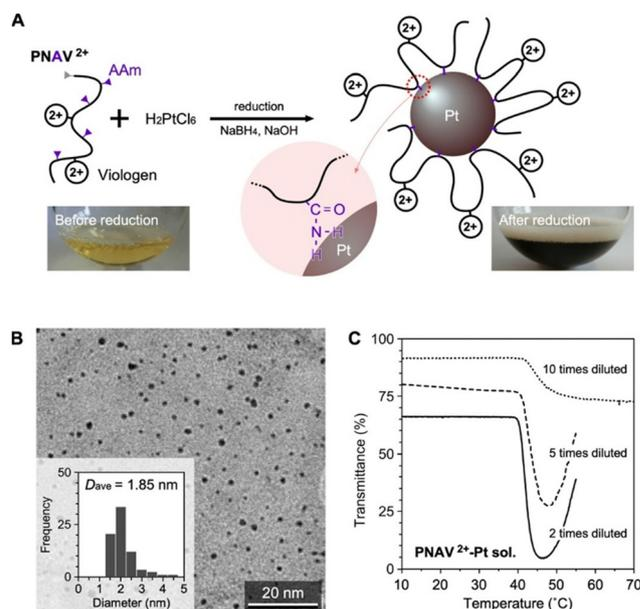
**Fig. 4** Preparation and properties of PNAV-conjugated Pt nanoparticles (NPs). (A) Synthetic scheme of PNAV-conjugated Pt NPs by the reduction method. Photos: before and after reduction of the aqueous mixture. (B) TEM image of PNAV-conjugated Pt NPs. Inset: Size distribution of the NPs. (C) Temperature dependence of the transmittances of the PNAV<sup>2+/+</sup>-conjugated Pt NP colloidal solution. Tris-HCl buffer solution (25 °C, pH 7.4, 500 mM);  $\lambda = 700$  nm.
