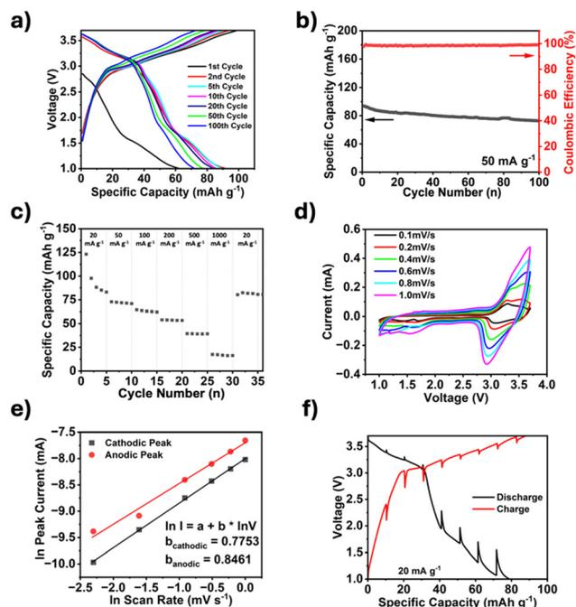
**Fig. 3** Electrochemical and kinetic tests on TPDA-ABDC. (a) Galvanostatic charge and discharge curves of select cycles at a 50 mA g<sup>-1</sup> current density, (b) cycling performance at a current density of 50 mA g<sup>-1</sup>, (c) rate performance test from 0.02–1 A g<sup>-1</sup>, (d) cyclic voltammetry at various scan rates, (e) plot of natural log of scan rate vs. natural log of peak current, (f) GITT with a 30 min pulse time at 20 mA g<sup>-1</sup> and 3-hour rest period.
