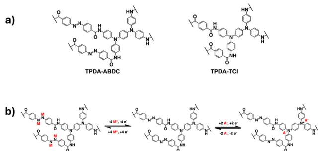
**Fig. 1** (a) The molecular structure of TPDA-ABDC and TPDA-TCl, (b) The proposed redox mechanisms for both functional groups of TPDA-ABDC, with M representing Na<sup>+</sup> cations, and A representing PF<sub>6</sub><sup>-</sup> anions.
