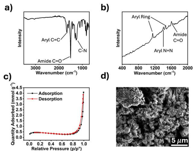
**Fig. 2** Characterization of TPDA-ABDC. (a) FTIR spectrum, (b) Raman spectrum, (c) N<sub>2</sub> adsorption/desorption curve, (d) SEM image of TPDA-ABDC.
