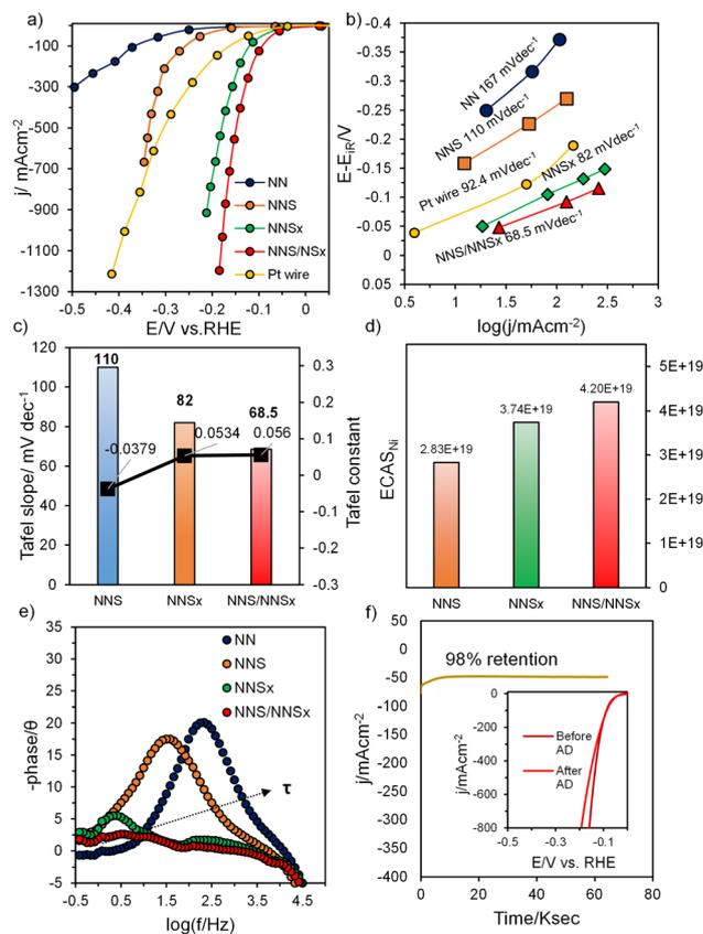
**Fig. 4** (a) HER SCV curves with 100% iR compensation; (b) Tafel plots derived from SCV (catalytic turn-over region) for NN, NNS, NNS<sub>x</sub> and NNS/NNS<sub>x</sub>; comparative bar diagram showing; (c) Tafel slope and Tafel constant; (d) ECAS<sub>Ni</sub> for NNS, NNS<sub>x</sub> and NNS/NNS<sub>x</sub>; (e) Bode-phase angle plot with time constant and (f) HER stability curve for NNS/NNS<sub>x</sub> with the inset showing before and after activity results.
