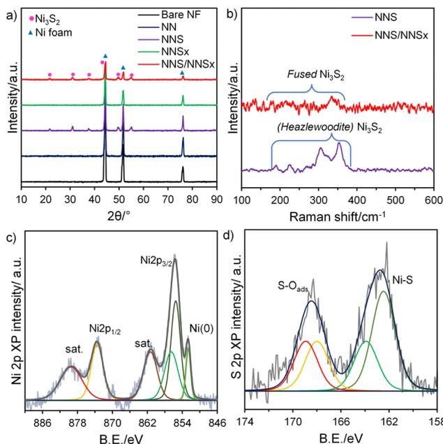
Fig. 2 (a) XRD pattern; (b) Raman spectra for different electrocatalysts; (c) core level XPS spectra of (c) Ni 2p and (d) S 2p for NNS/NNS<sub>x</sub>.
