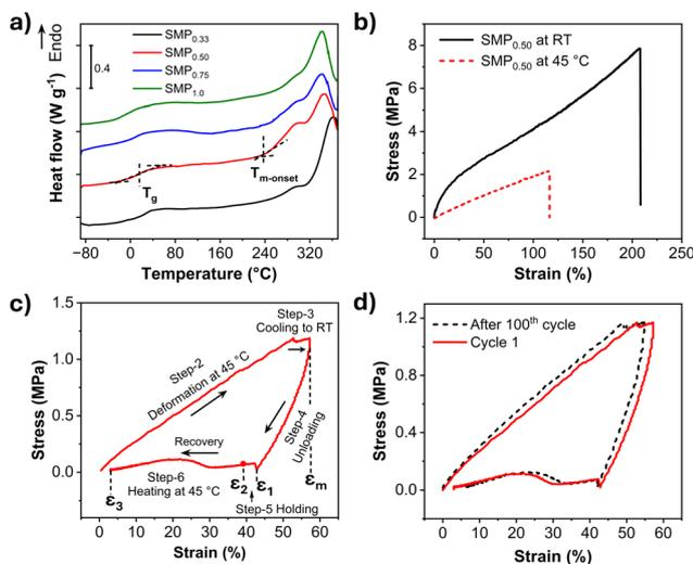
**Fig. 3** (a) DSC analysis of 3D-printed SMP<sub>0.33</sub>, SMP<sub>0.50</sub>, SMP<sub>0.75</sub> and SMP<sub>1.0</sub>. (b) Tensile testing of SMP<sub>0.50</sub> at RT and 45 °C. (c) stress-strain plot for a thermomechanical test cycle, and (d) cyclic thermomechanical test comparison of a specimen of SMP<sub>0.50</sub> after 100 cycles of shape transformation cycle.
