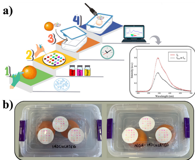
Fig. 2 (a) Steps for sensing by the fluorescent array: (1) inoculation of oranges with Penicillium digitatum or s.d.w., (2) drop casting of fluorescent probes onto the polyamide support, (3) positioning of oranges and the sensor array into the box, (4) analysis of fluorescent probes by the optical fibre. (b) Photographs of the packaging containing the oranges: “inoculated” on the left and “non-inoculated” on the right.
